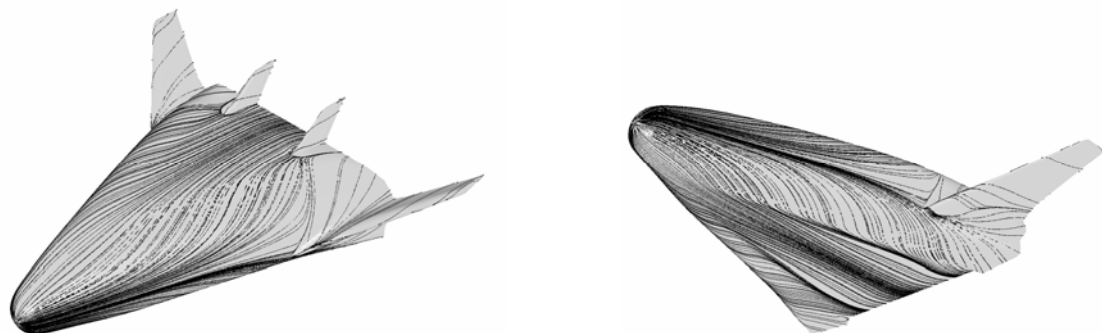
(b) Surface streamline patterns for the X-33 configuration at the peak laminar heating point ( M_\infty=10 , \alpha=20^\circ )
